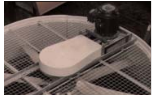
▲ Motors, drives, pumps are all located externally for ease of operator access. No need to enter confined spaces to adjust belts and so on.
