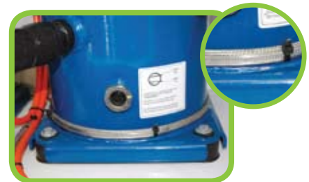
Sump heater on compressor for reliable cold morning starts
